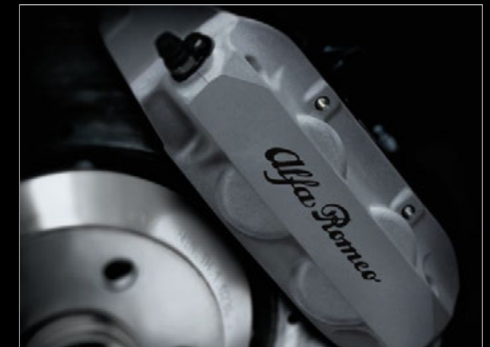
Dual-cast, cross-drilled, self-ventilated, 305- x 28-mm front discs with Brembo® fixed 4-piston calipers
